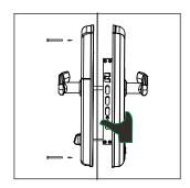
6.Use one hand to press front faceplate against the door, fix back faceplate with 2 screws.
