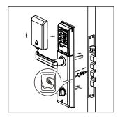
5.Take out battery cover, connect cables of front and back faceplates, and makesure knob is fixed in correct direction.
