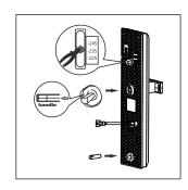
1.Place the template on the door. According to the template, mark the holes on the door with a pencil.
