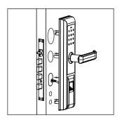
4.Install front faceplate, making sure different parts go into correct holes.
