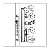
10.Test the installation by inner handle, knob, mechanical key, fingerprint, password and reading card.
