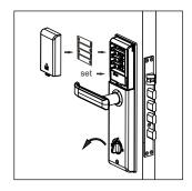
8.Install the battery box and batteries, test the deadbolt.
